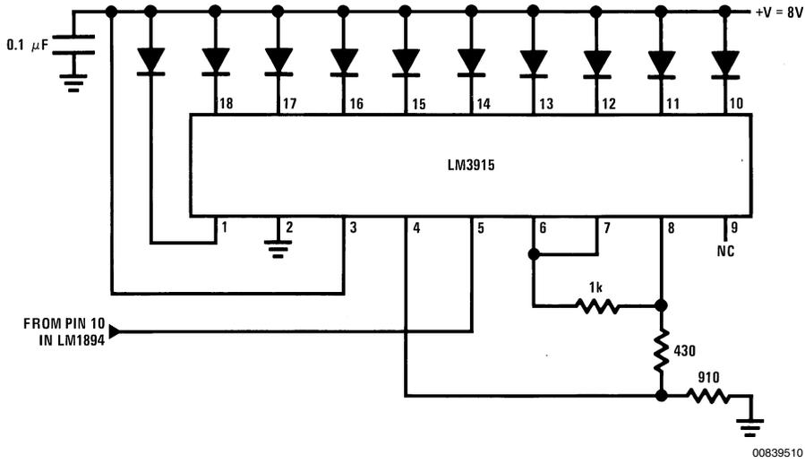
FIGURE 10. Bar Graph Display of Peak Detector Voltage
