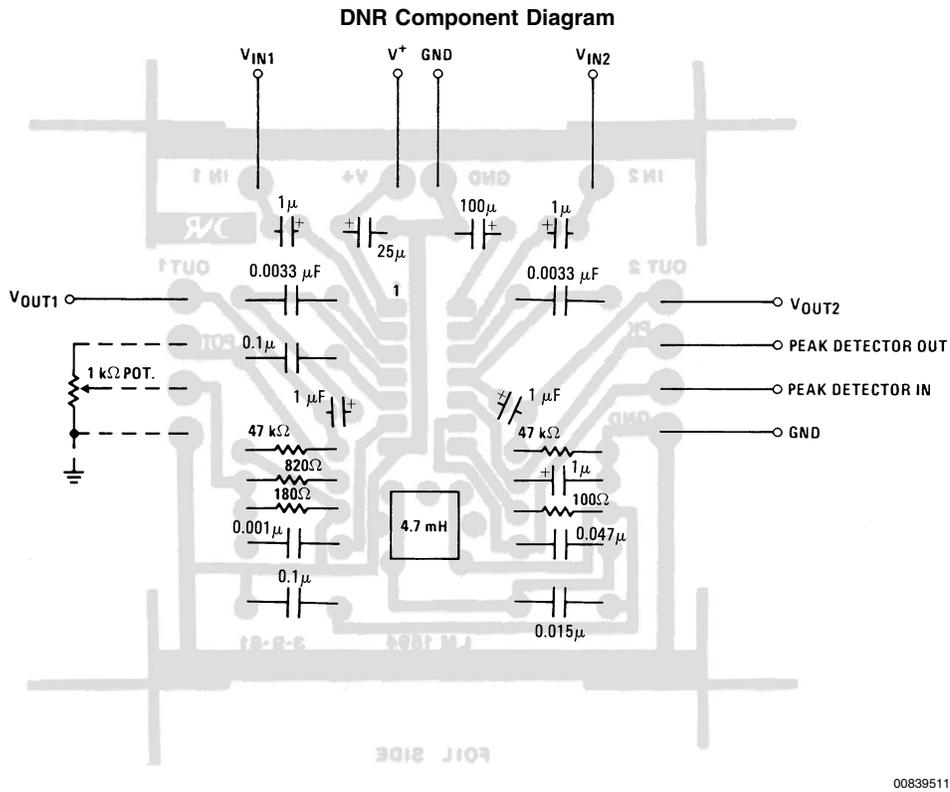
FIGURE 11. Printed Circuit Layout
